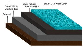
Our poured-in-place rubber surfacing is a two-layer system consisting of a cushioned base, composed of a high quality recycled rubber, and a top surface made of rubber/EPDM granules. We offer a wide array of colors that can be mixed or used side by side.
